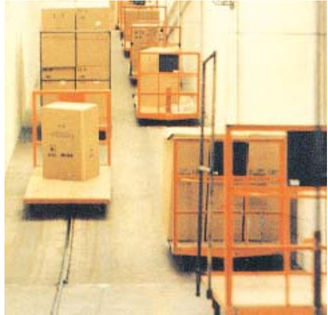
Towline conveyor system for carton transport
