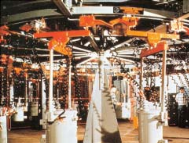
Power-and-free conveyor system
